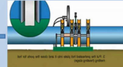
3. Put the preheated hot plate into it and close the ports for hot melting (heating stage)
