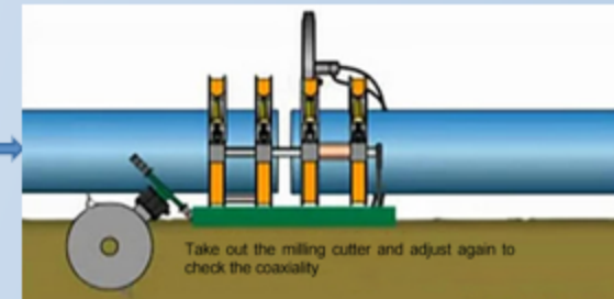
Take out the milling cutter and adjust again to check the coaxiality
